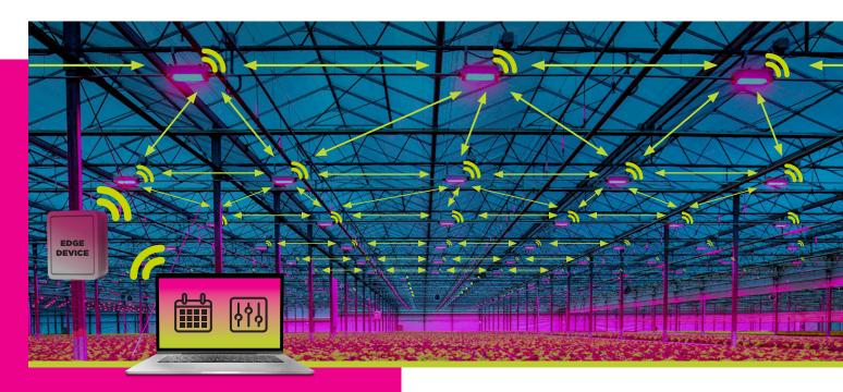
The Oreon LED Control Center (OLCC) enables the grower to control their assimilation lighting with unmatched precision. The lighting installation is dynamically controlled by a fine mesh network, which is formed by all the lamps in the greenhouse or cultivation area. This allows the grower to respond to fluctuating light needs and energy rates. The result is the exact desired amount of light at any time or place at the lowest possible cost.
